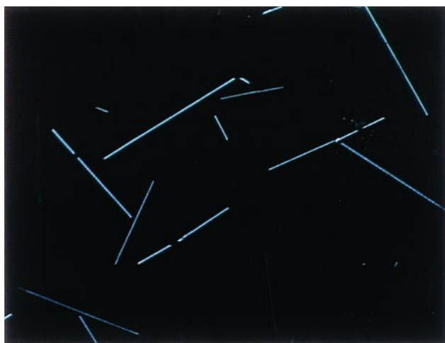
Plate 2 Micrograph of the mesophase of 4b at room temperature after cooling from the isotropic phase (crossed polarizers)
