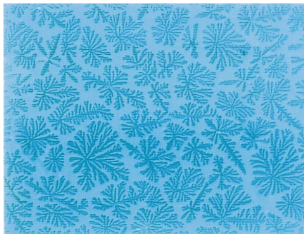
Plate 3 Digitate stars observed in the mesophase of 4a at 85 °C upon cooling from the isotropic phase (parallel polarizers)
